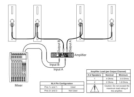
In the PSAT1 both the LF and HF drivers are connected to pins 1+/1– of the NL4 connector.
